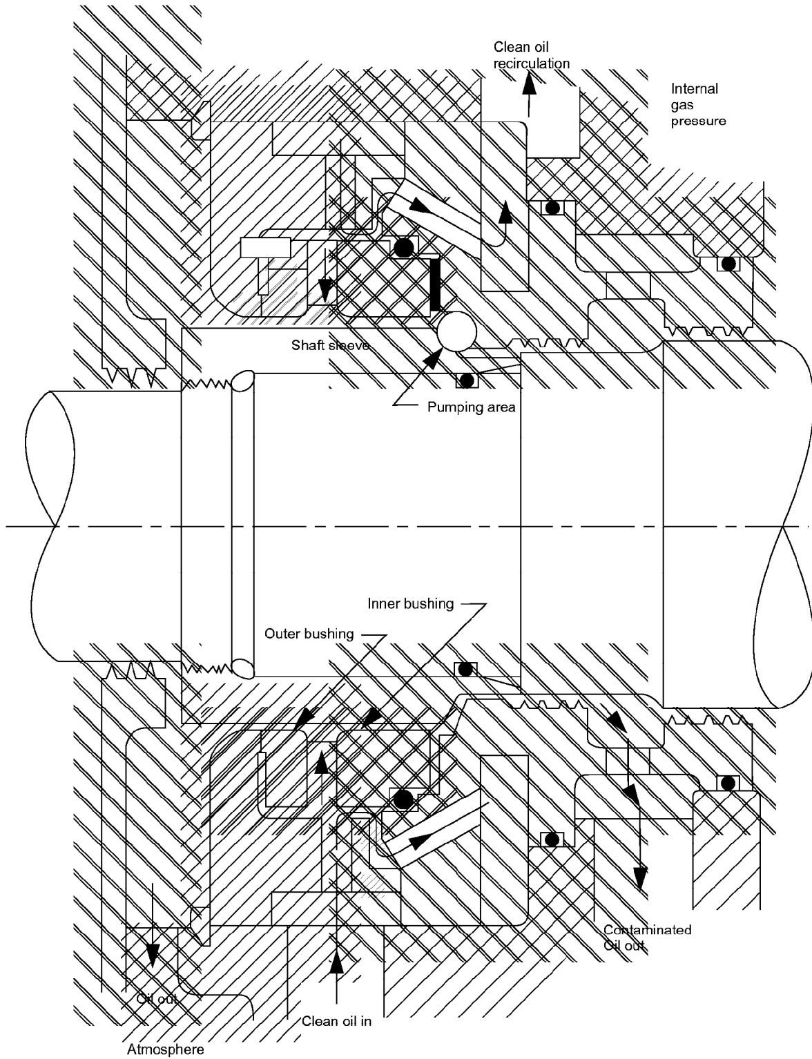
Figure 1.C-5—Liquid-film Shaft Seal with Pumping Brush
